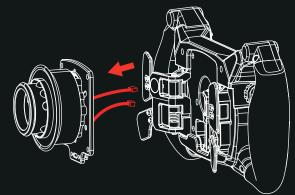
Remove the QR, the panel and the socket. (Note: Both cables need to be uplugged gently
