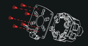
Install the Maglink panel on the wheel and secure with the screws removed from step 2.1.
