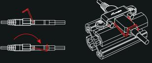
Use the snap-on to secure the connector.
